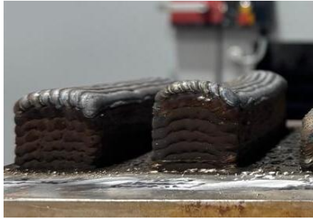
No start stop ramp up procedure
