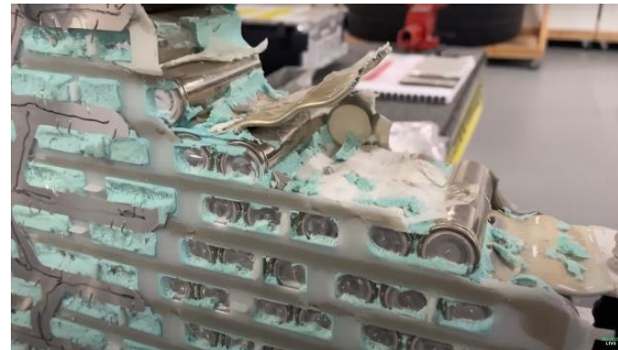
Tesla Model S composed of 4416 cells held together with strong adhesive
