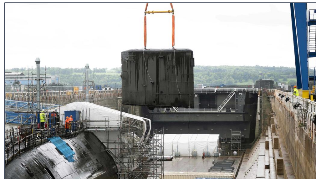
Decommissioned submarine 'Swiftsure' has its fin cut and removed (June 2025)
