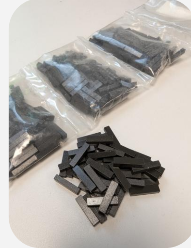
Epoxy coated motor magnets
