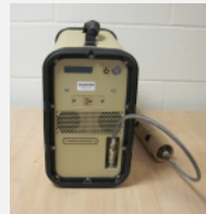
250 W SOFC operating on propane
