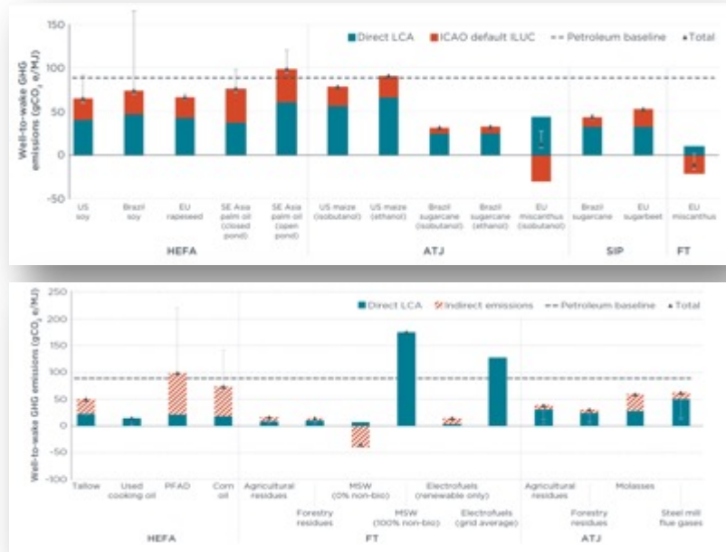
Well-to-wake GHG emissions for sustainable aviation fuels relative to petroleum jet fuel baseline (top – crop based, bottom – waste based)
