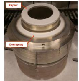
Mockup Upper sleeve removed
