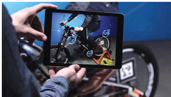
Figure 3. PTC outfitted a Santa Cruz mountain bike with sensors that connect to an NI myRIO system which measures parameters such as fork travel, wheel speed, and steering angle. The data gets beamed to the PTC ThingWorx platform in the cloud to create a digital twin of the bike that displays in real time on an iPad or similar platform (PTC, 2016).
