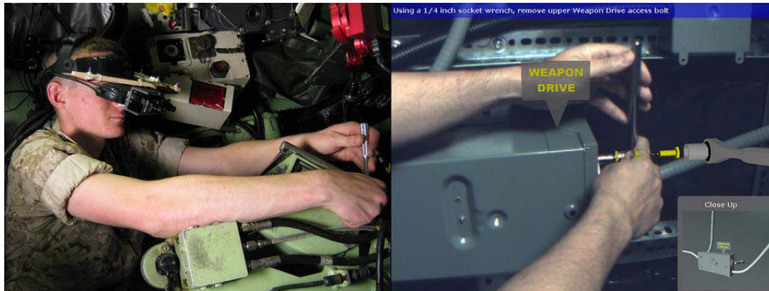
Figure 4. A mechanic wearing a tracked head-worn display performs a maintenance task inside an LAV-25A1 armoured personnel carrier (Henderson & Feiner, 2016).
